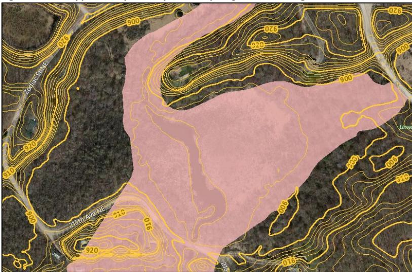
3.13 The regulatory limits of the district boundaries shall be further extended outward based on the horizontal extension of the Regulatory Flood Protection Elevation (RFPE) (Figure 2).
